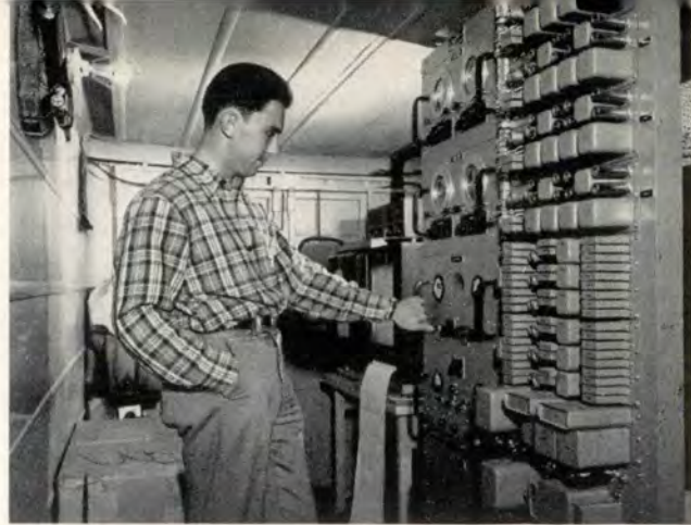
Electronic devices check the mountain wave's effect on the sailplane, and record a "play-by-play" account.
