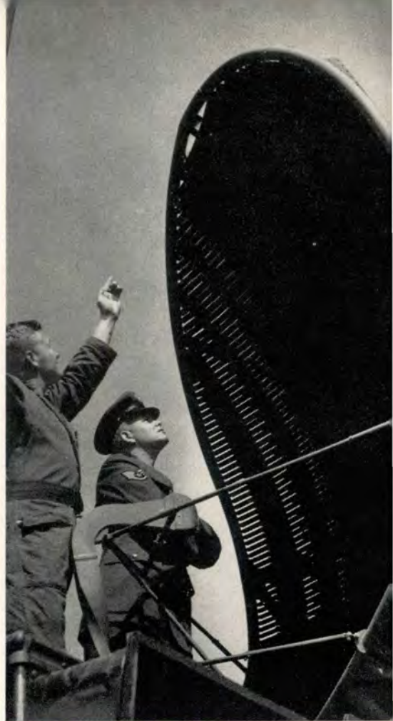
Refinements to GCA equipment have greatly increased the effectiveness and range of radar operations. Shown here is the newer "dish" type antenna of the CPN-4 unit.
