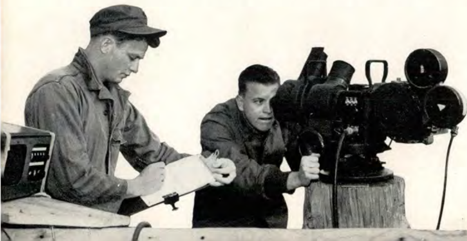
Air currents were investigated by taking time-lapse motion pictures from the ground and correlating them with sailplane recordings.
